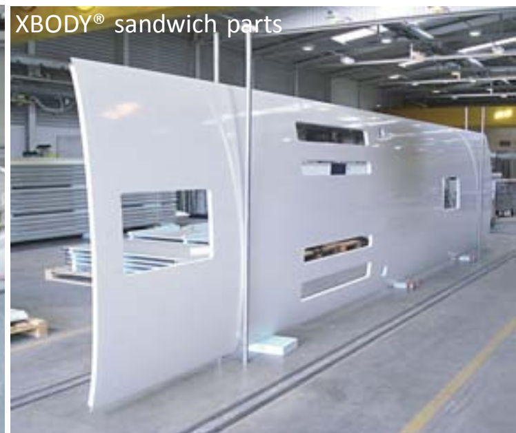
INNOCAB® Front Cabin sandwich-panel structures made of fiber-reinforced plastic
