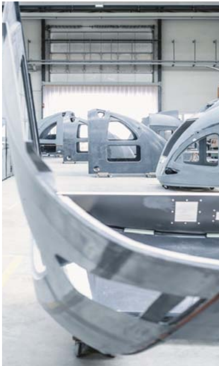
INNOCAB® Front Cabin sandwich-panel structures made of fiber-reinforced plastic
